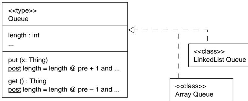
**Figure 6.4** Different implementations of the same type model.
