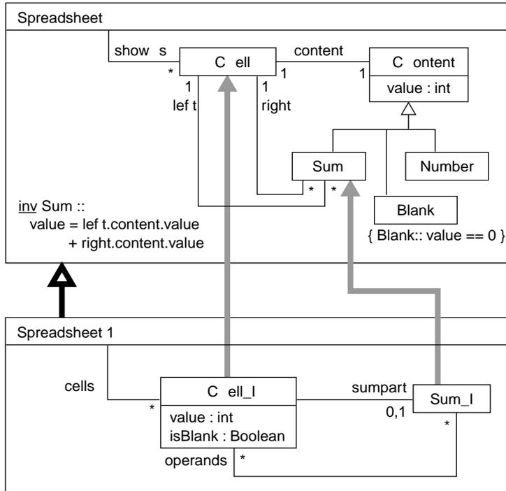
**Figure 6.22** Spec and code, showing main correspondences.
