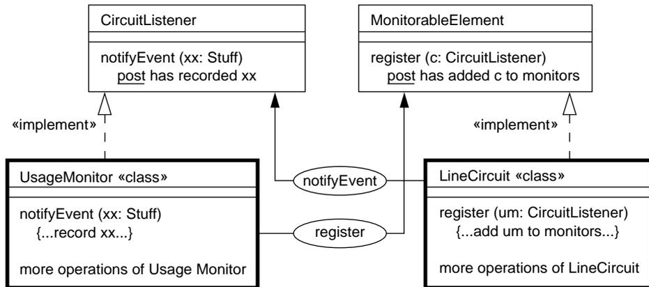
**Figure 7.14** Decoupling via types.
