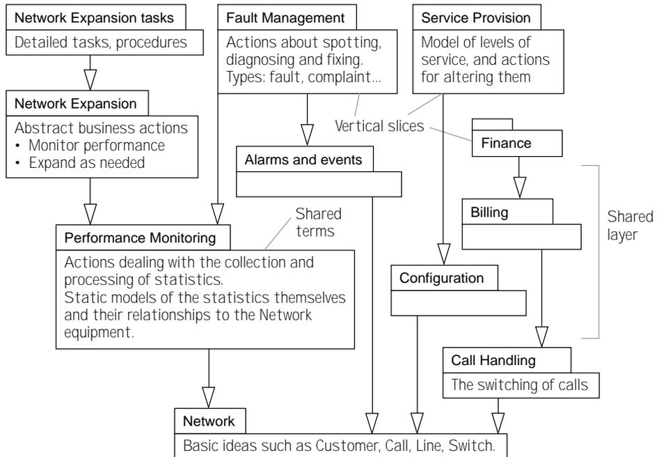
**Figure 7.10** Packages segment vertical slices from a common base.
