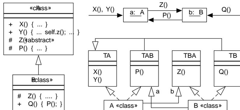
**Figure 11.12** From inheritance to type-based composition.
