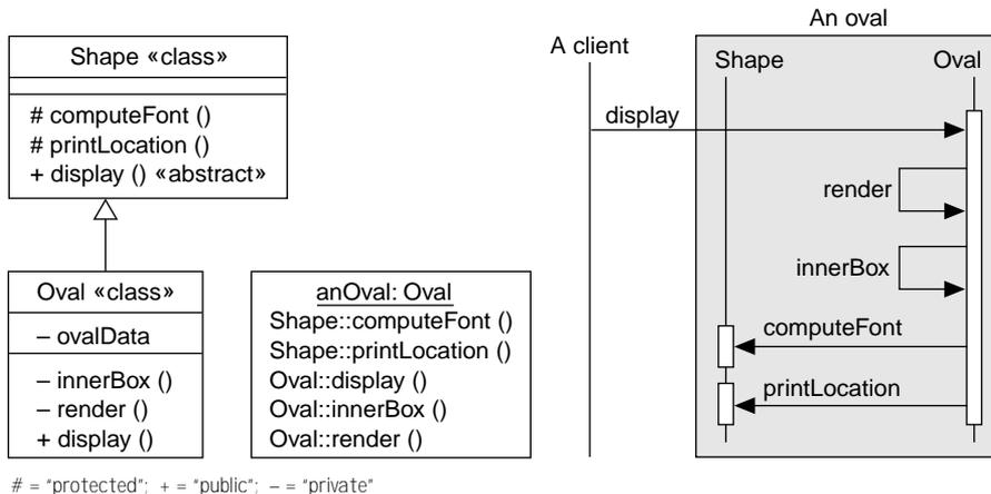
**Figure 11.5** Inheritance design and enhanced interaction diagram.
