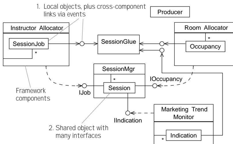
**Figure 11.11** Two alternative ways to compose code frameworks.
