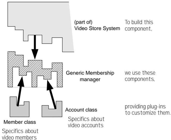
**Figure 11.4** Using lower interfaces to customize a component.
