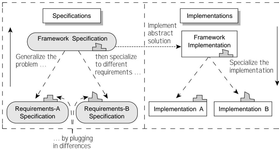
**Figure 11.8** Frameworks for specification versus implementation.
