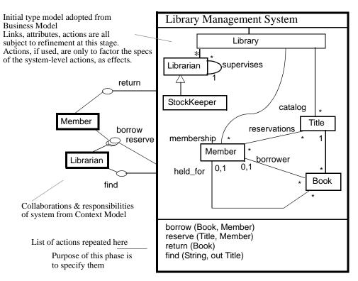
**Figure 15.4** Initial type model derived from business model
