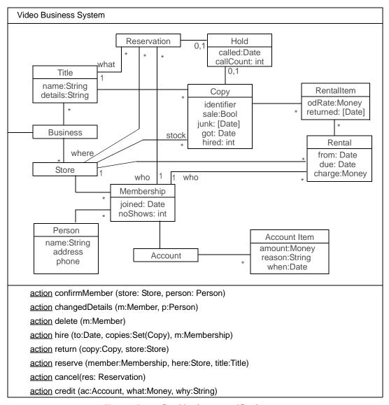
Figure 15.20 Combined type specification
