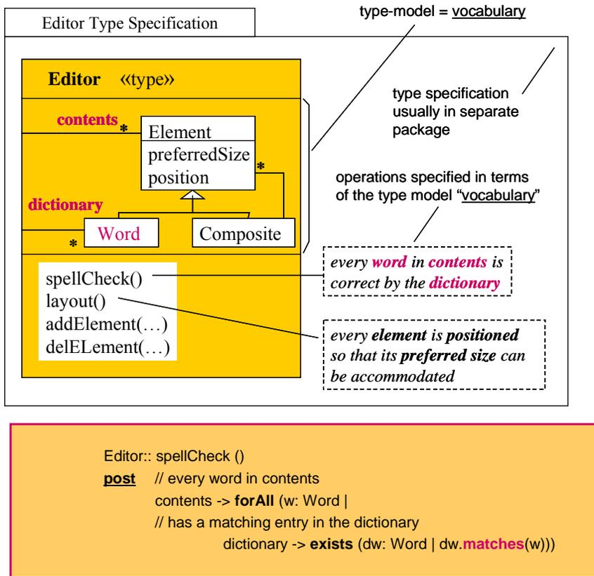
Figure 4 Model-based specification
